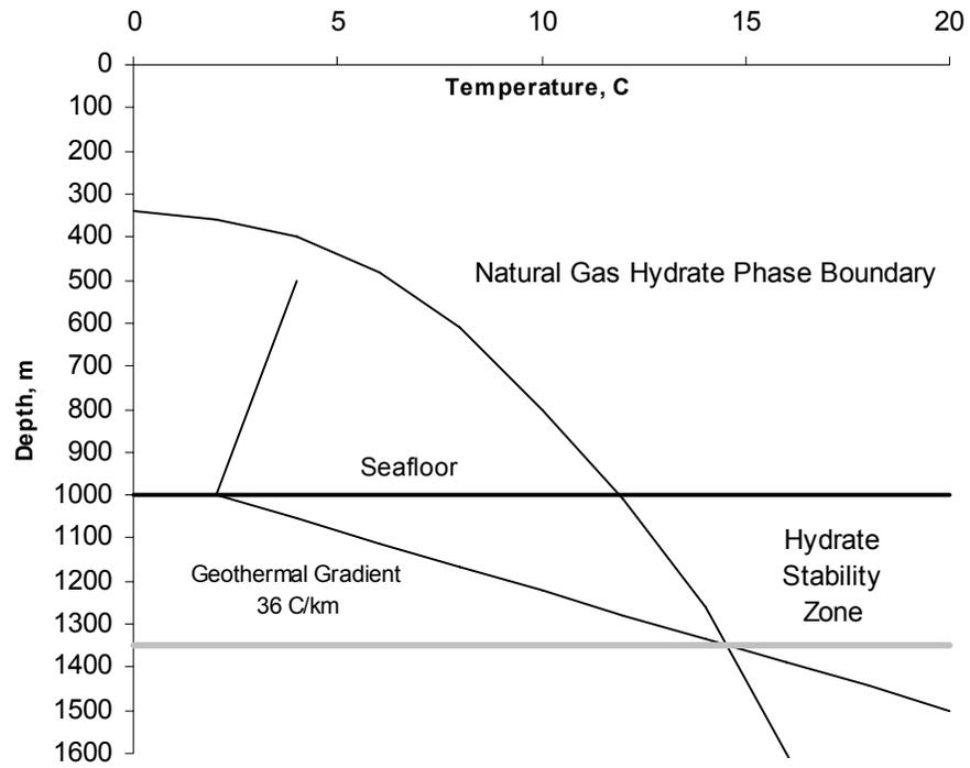
**Figure 1. Position of the hydrate stability zone in the upper sediment (Kvenvolden 1993). Geothermal heat rising from below establishes the base of Hydrate Stability Zone (HSZ) as phase boundary limit. Representative hydrothermal and geothermal temperatures shown.**
