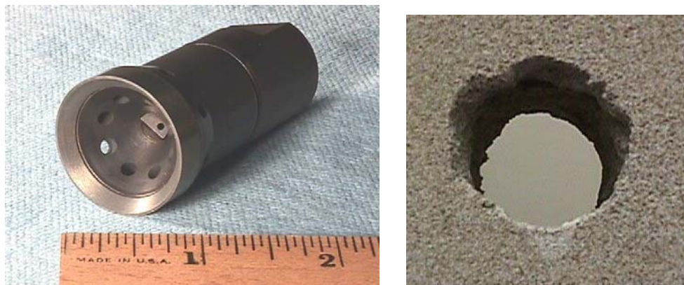
Figure 10. Compact jet drill and 1-1/4" hole drilled in Wilkeson sandstone at 70 MPa
