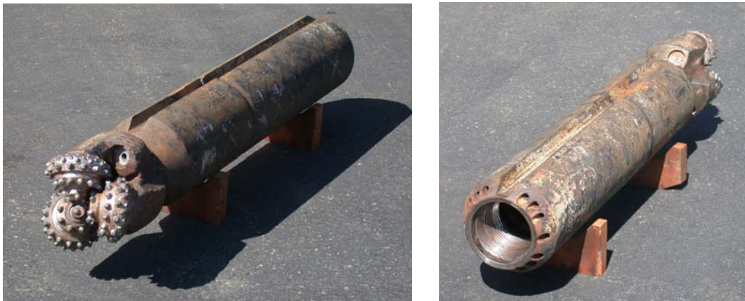
Figure 2. Hydraulic pulse tool housing with high-speed flow courses.
