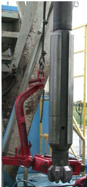
Figure 2. Hydraulic pulse tool housing with high-speed flow courses.
