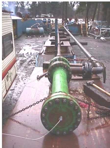
Figure 4. Second generation hydraulic pulse tool with high-speed flow course housing and sweep mechanism.
