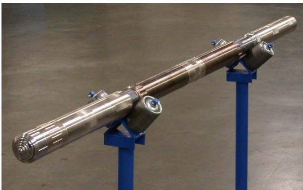
Figure 15. Downhole intensifier BHA including gas separator, downhole intensifier and high-pressure rotary jet mill.
