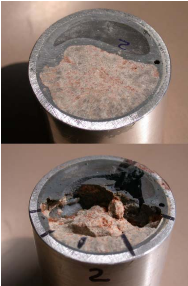
Figure 2. Barite sample before and after jetting at 90 MPa (13,000 psi). Dark material is epoxy.
