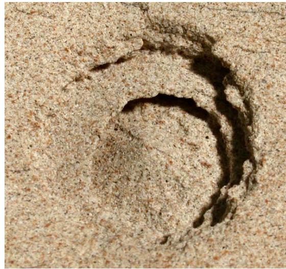
Figure 17. Cutting pattern in sandstone produced by six-jet high-pressure milling head.
