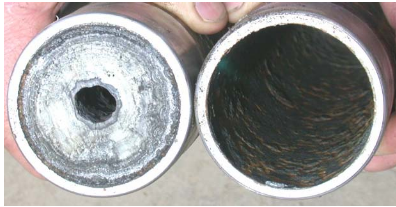
Figure 11. Heavy carbonate scale milled at 1 m/min with GS-RJMT at 34 MPa differential pressure, 90 lpm water, 15 scmm nitrogen.
