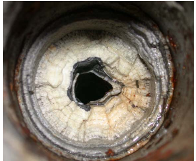
Figure 22. Six-jet milling head cutting patterns in heavy carbonate scale.
