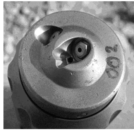
Figure 9. Jetting head showing forward facing water jet nozzles and gas ports after service.
